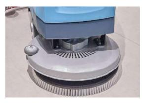
For safety reasons: Leave or service the machine, park on a level surface, turn off the machine and pull out the key,Start the machine, lift up the brush tray assembly (do not start the washing function), lift the side guard plate and open it as shown in the picture, then move the
